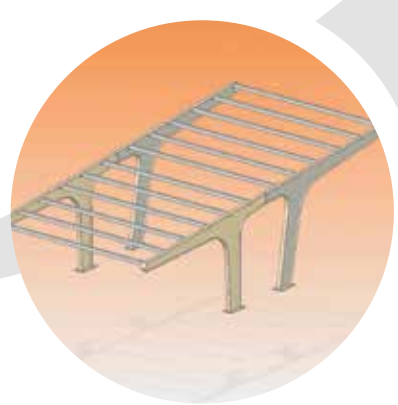
Carport for 4 parking lots with 2 m wide footpath is suitable for installation of 36 PV modules
